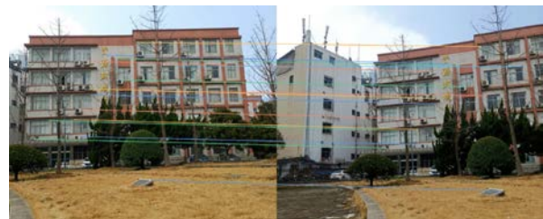
Figure 5 Example of matched features using SIFT features in two photos with different view angles.
